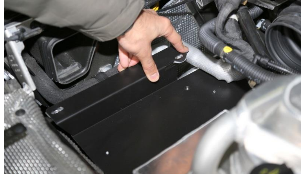
18. Take the smaller heat shield and lower it into position on the left side as shown.
