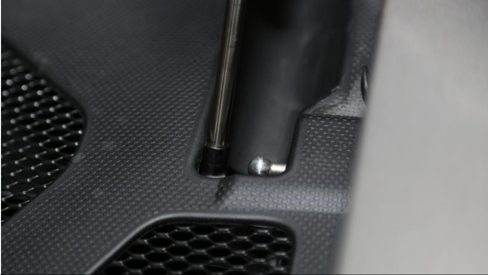
5. Once the clip has been unlocked – push the strut out from the ball joint.
