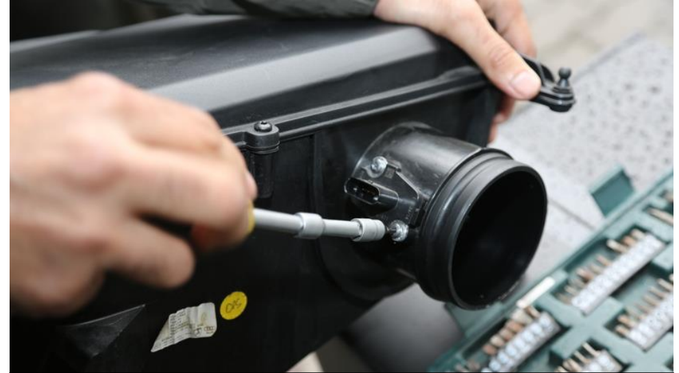
14. Remove the MAF sensors from the original airboxes. They are held in place with 2 screws.
