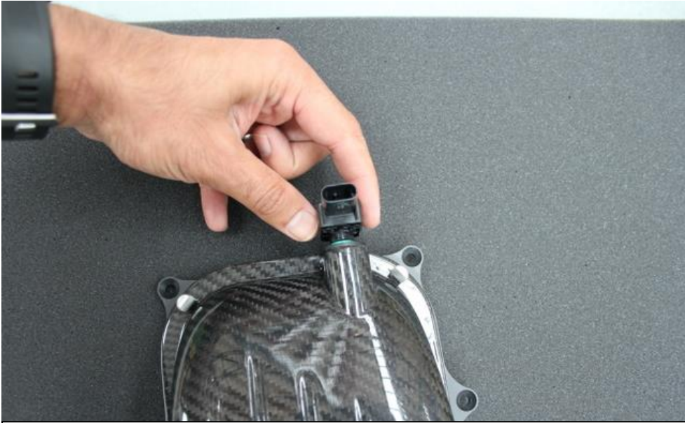
9. Install both MAP sensors into the carbon airbox lids. Push them in vertically and then rotate 90 degrees. It may help to slightly lubricate the green O-rings on the sensors.
