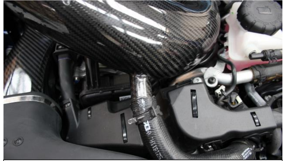
23. Take the Left side airbox lid and push the breather pipe into the front.
