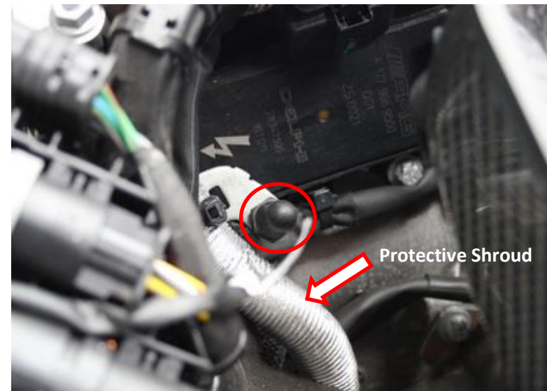
18. The rubber needs to locate onto this mount at the back of the engine. Please rotate the mount on the airbox so that it lines up with the silver protective loom shroud shown.
