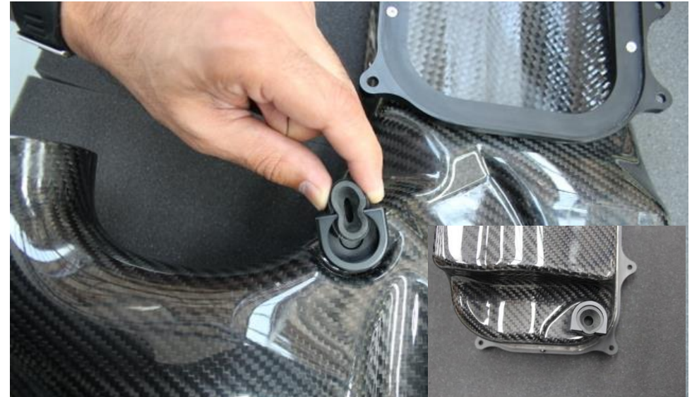
16. Push the rubber mounts into the mount holders on the carbon airboxes. There are 4 positions. One mount on each carbon piece. They can be pinched and pushed into the holders
