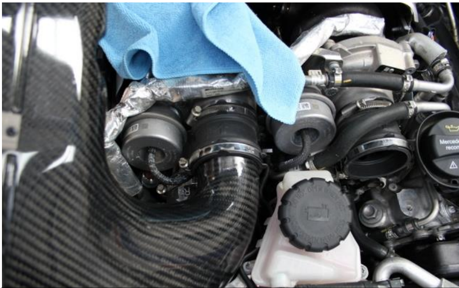
24. Push the outlet of the lid into the rubber coupler.
