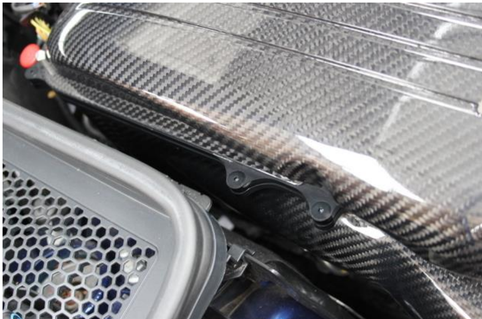
28. Secure the airbox with the supplied countersunk screws. Screws only need to be finger tight – do not put excess force on them.
