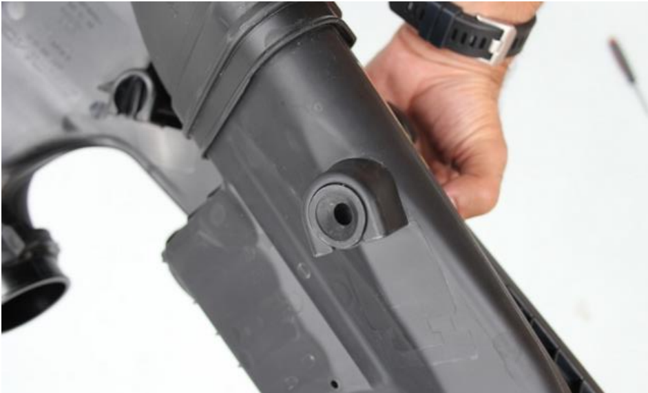
15. Remove 4 rubber mounts from the stock airboxes.
