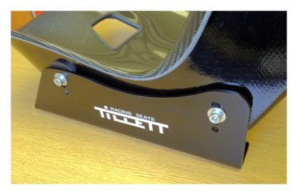
Make sure that high quality 12.9 strength M8 bolts are used for all mounting points and we recommend a torque setting of 35nM when fitting the bracket to the side mounting points.
