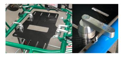
Remove the coned 18mm thick diameter spacer to lift seat above the lower level of tubes
