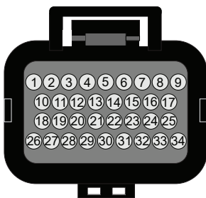
Nexus T2/T1 ECU harness connector pinout Wire side view
